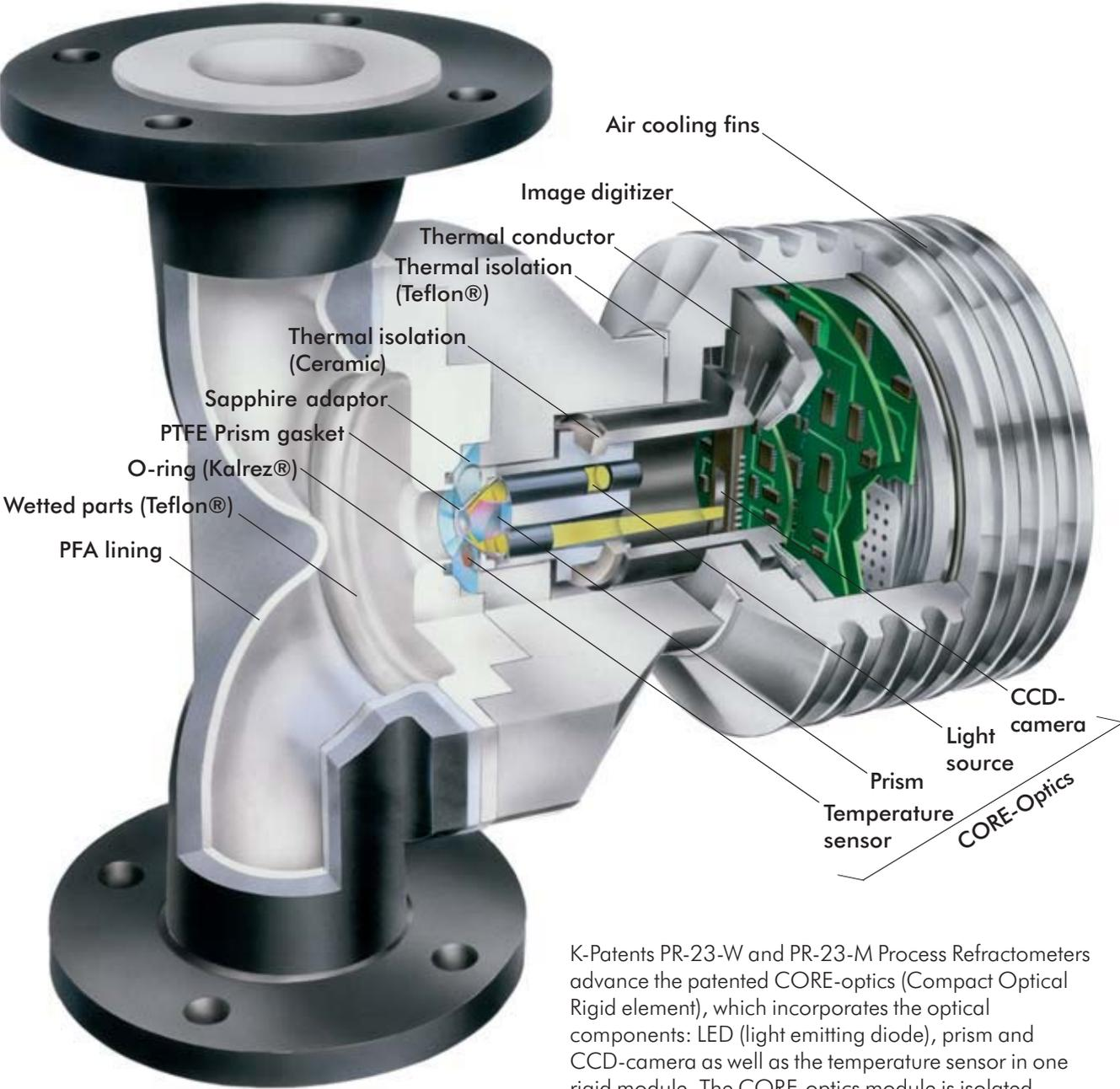
K-Patents PR-23-W and PR-23-M Process Refractometers advance the patented CORE-optics (Compact Optical Rigid element), which incorporates the optical components: LED (light emitting diode), prism and CCD-camera as well as the temperature sensor in one rigid module. The CORE-optics module is isolated from the sensor body and therefore external forces like pressure, flow and temperature changes do not influence the measurement.
