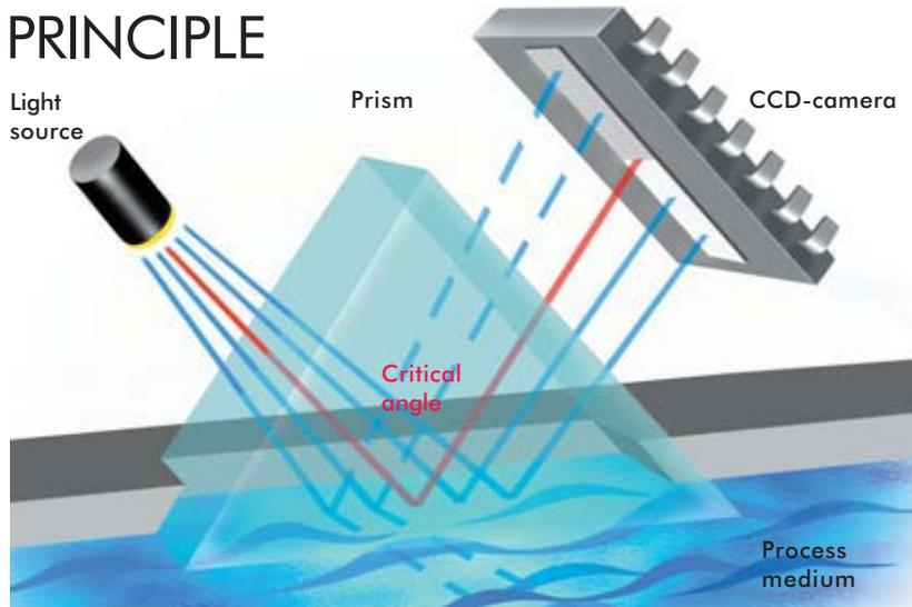
The light source sends light against the interface between the prism and the process solution, where the rays meet the surface at different angles.
