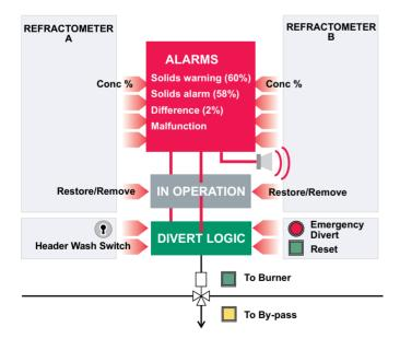
The divert decision is controlled by the divert control unit. The built-in logic provides three levels of decision rules for tight control.
