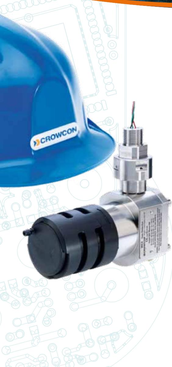
IREX is an innovative infrared (IR) flammable gas detector designed specifically to directly replace pellistor (catalytic bead) type flammable gas detectors. IREX operates from control systems designed solely for use with pellistor-based gas detectors: it produces a mV Wheatstone Bridge type signal (as per a pellistor) and operates from as little as 2.9Vdc. IREX is supplied with an M20 type fixing enabling originally installed detector junction boxes and cables to be retained.
