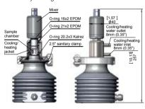
Mini flow cell PMFC for low volume pilot processes:
