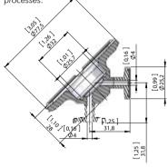
Indicating transmitter DTR in stainless steel enclosure:
