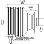
Laboratory test cuvette LTC for off-line laboratory testing:
