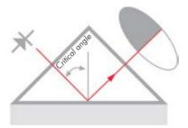
A digital CCD-camera detects the optical image and the shadow line. The camera transforms the optical image point-by-point to an electrical signal. The exact shadow line position is located and the refractive index  $n_{\rm p}$  is determined.
