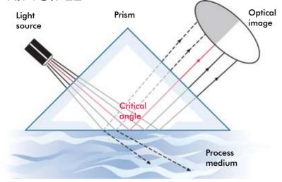
The light source sends light against the interface between a prism and the process solution, where the rays meet the surface at different angles.
